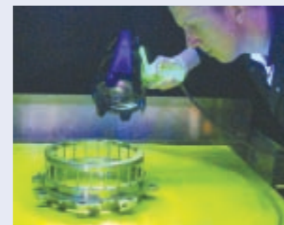
Amfin's magnetic particle inspection unit in use on gas turbine bearing housing.
